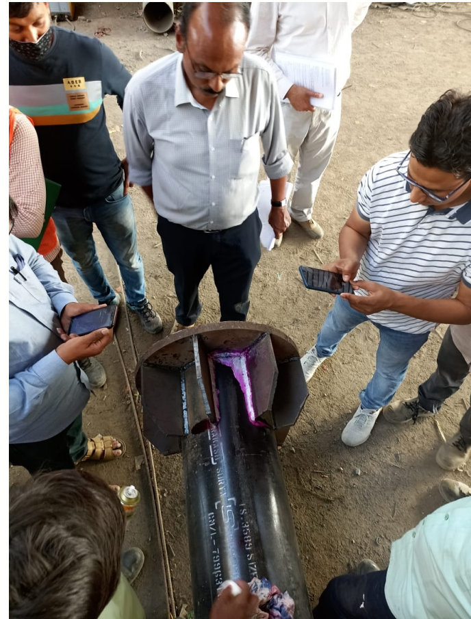
Dye penetration test conducted
