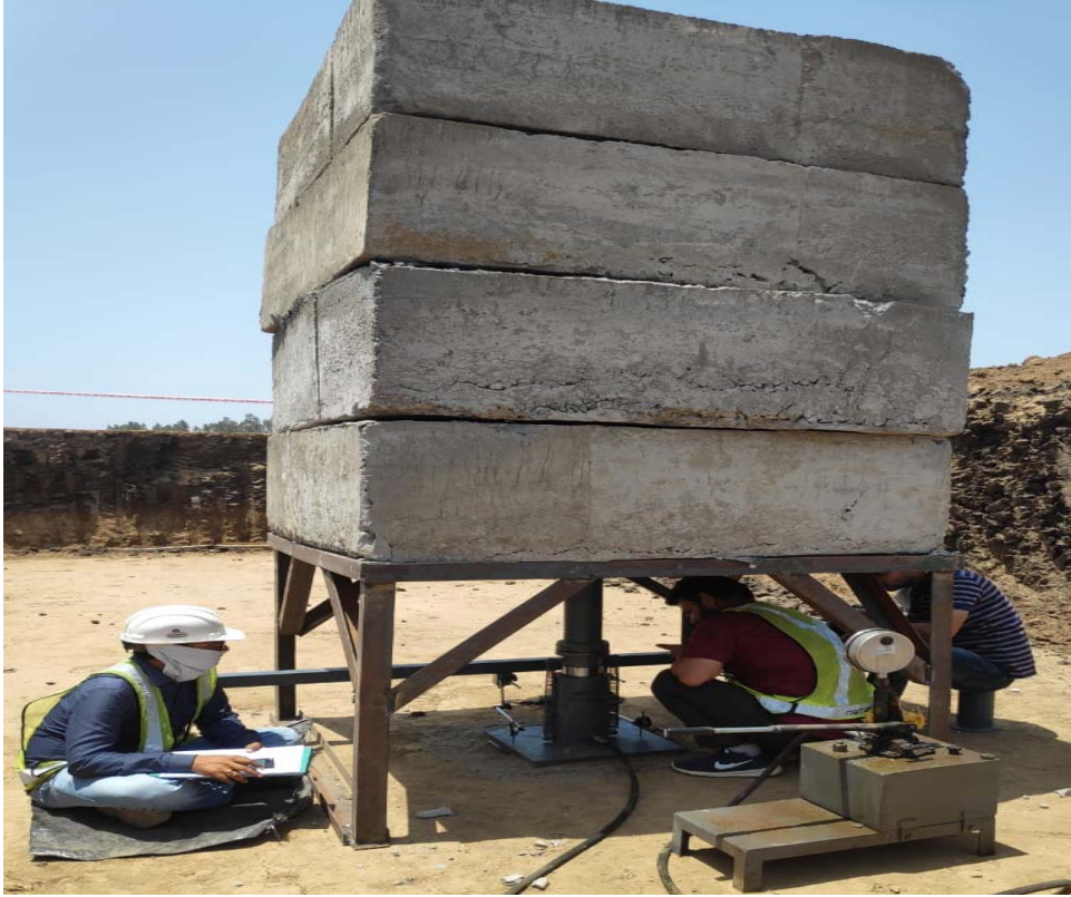
Plate Load Test at 322+450
