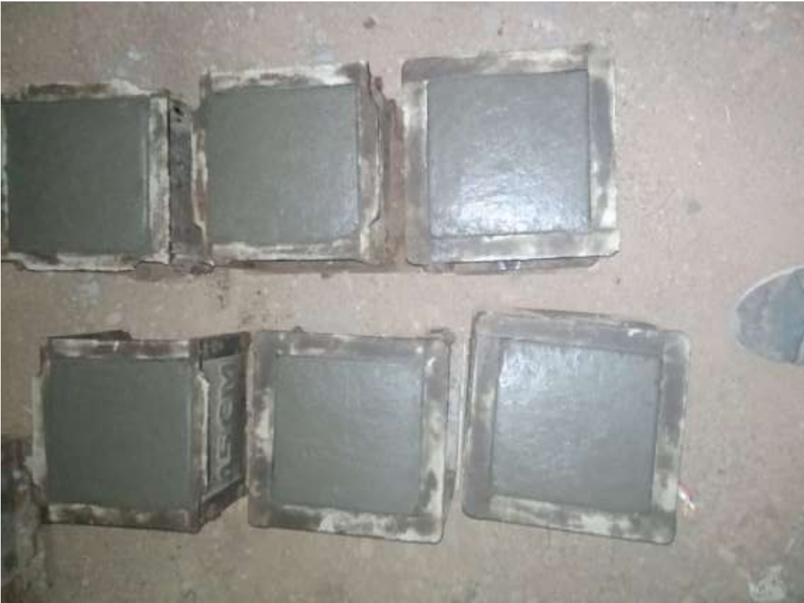
Cube casted for Trail mix design of M-40
