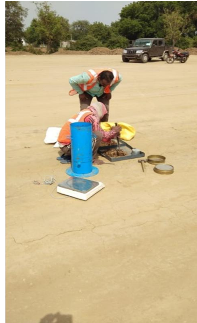
Ch. 345+500 - FDD Testing of Embankment
