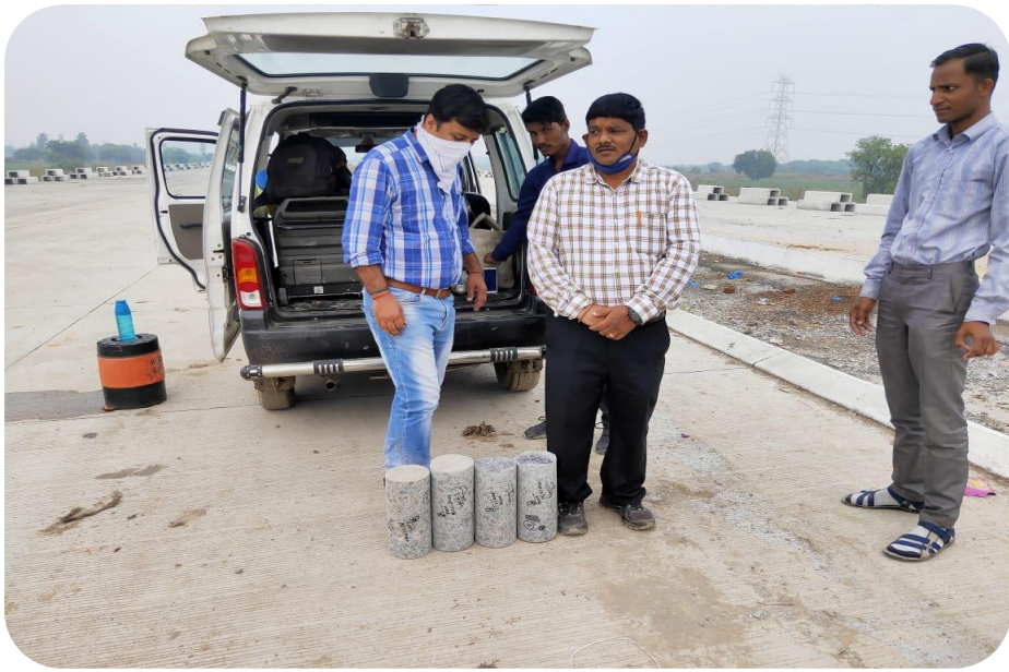
CORE CUTTING SAMPLE OF PQC AT CH 339+500
