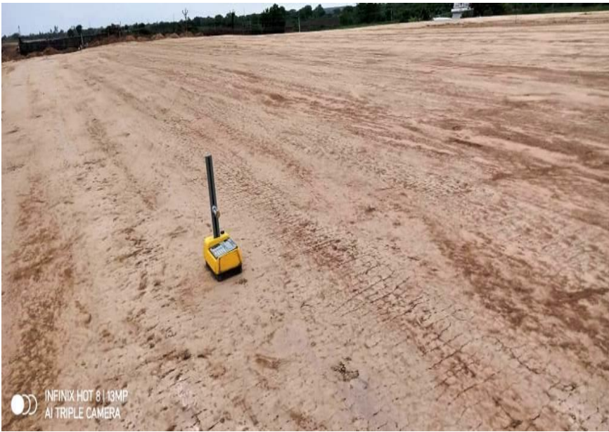
329+410 TO 329+550 RHS EMBANKMENT TOP FDD CHECKING
