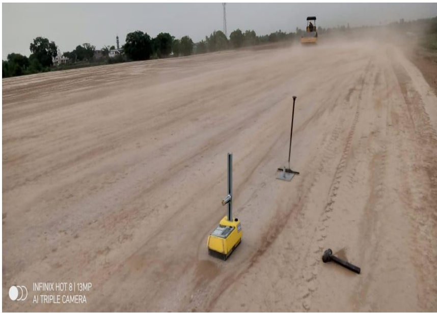
329+410 TO 329+550 EMBANKMENT FDD CHECKING
