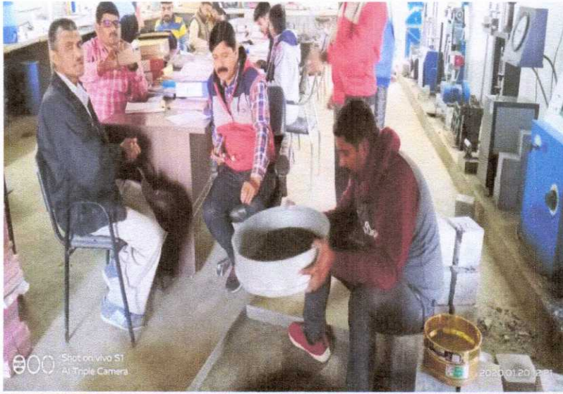
GSB GRADATION TEST FOR SITE SAMPLE FOR CH. 337+960 TO 338+160
