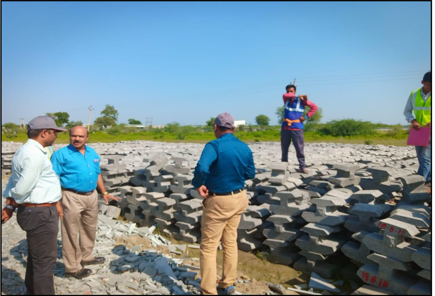
Sampling of RE Wall Blocks by Team Leader at Eartcon Plant
