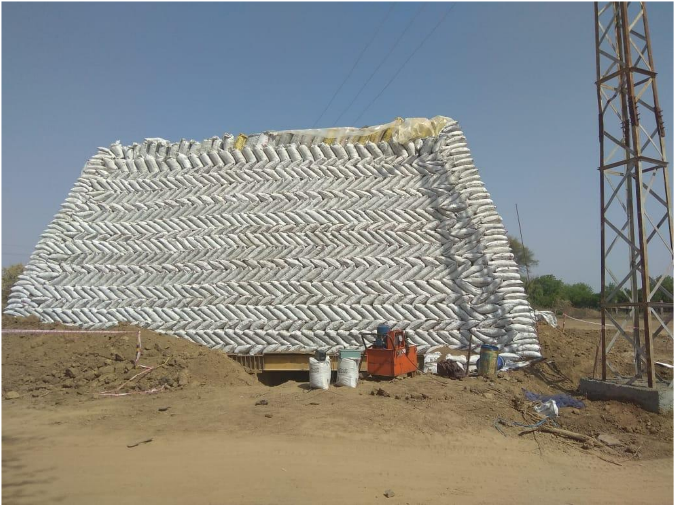
Pile Load Test on Test Pile @ Ch.36+070 (MJB)
